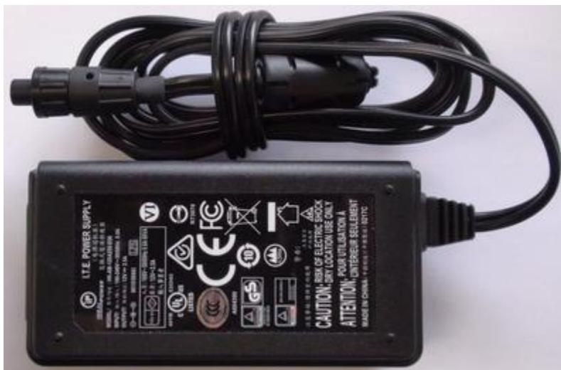
Figure 2: 12Vdc 2.5A 100-240VAC Power Adapter
