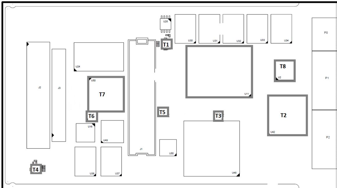
Figure 2: BM Temperature sensor locations
