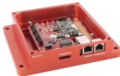
Figure 4: Enclosure used for accommodating the FM191 and EMC2-DP
