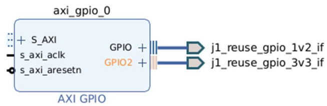
Figure 16 – Selecting axi_gpio for J1 board interface
