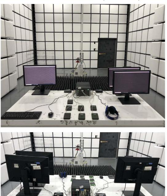
**RADIATED EMISSION TEST (Above 1GHz)**
