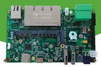
The RTSO 6003/6003E board is an industrial-grade board for Nano/Xavier NX/TX2 NX/Orin NX. It has abundant interfaces, low power consumption, and high security level, which can meet various harsh conditions.
