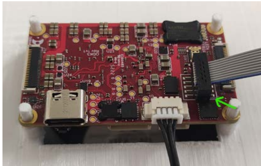
Figure 7 - JTAG In on the VCS 3 Note Pin 1
