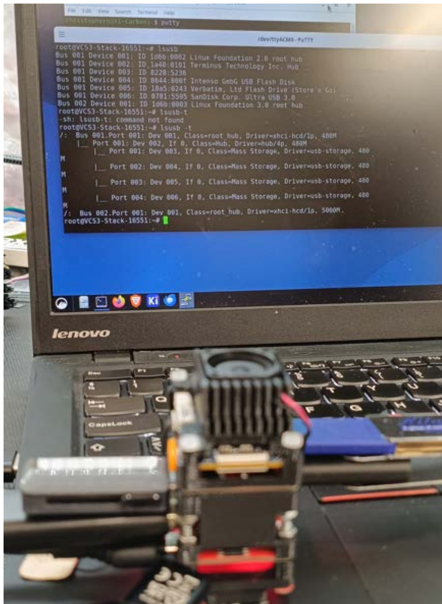
Figure 12 VCS3-Stack with 4x USB memory sticks connected and detected
